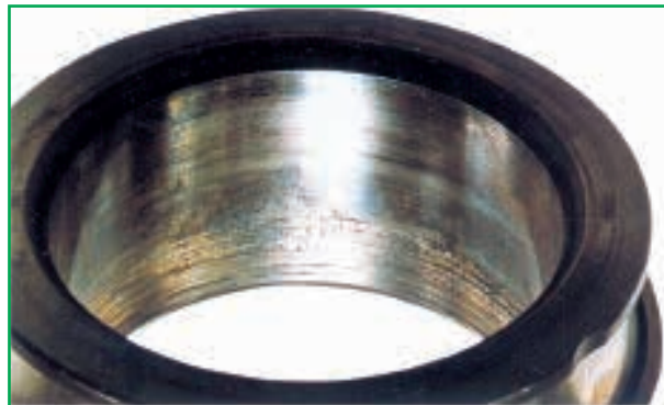
Fig. 19 Part: inner ring of a spherical roller bearing Symptom: creep accompanied by scoring of bore surface Cause: insufficient interference
