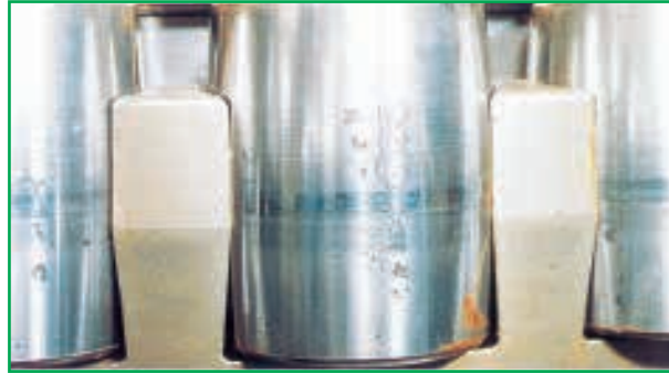
Fig. 7 Part: rollers of a spherical roller bearing Symptom: pit-shaped rust on rolling contact surface. Corroded portions Cause: moisture condensation during storage
