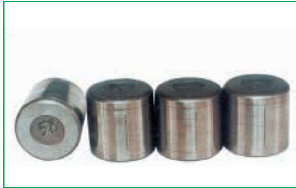
Fig. 25 Part: rollers of a cylindrical roller bearing Symptom: axial scratches on rolling surface Cause: inclination of inner and outer rings during mounting
