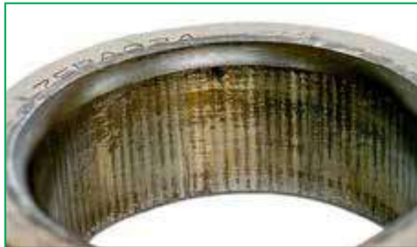
Fig. 17 Fretting corrosion on entire surface of inner ring bore
